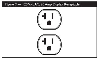
Use each receptacle to operate 120 Volt AC, single—phase, 60 Hz electrical loads requiring up to 2,400 watts (2.4 kW) at 20 Amps of current. Use cord sets that are rated for 125 Volt AC loads at 20 Amps (or greater).
